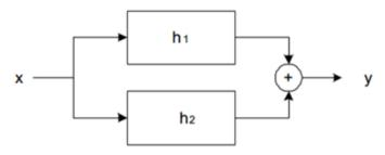
The impulse response  $h_1[n]$  is given as  $h_1[n] = \delta[n] + \delta[n-1] + \delta[n-2]$ . We feed the system with the discrete time signal  $x[n] = \delta[n] + \delta[n-2]$ , and observe the output
